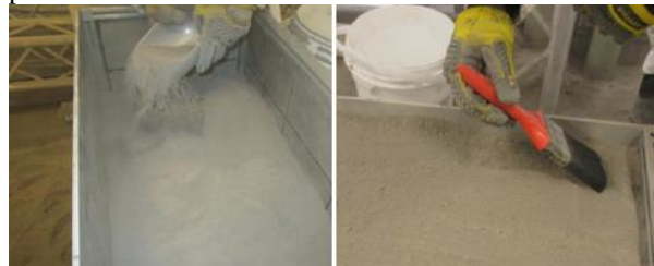
Figure 2: The ‘snowing’ technique produces the most consistent geotechnical properties.
